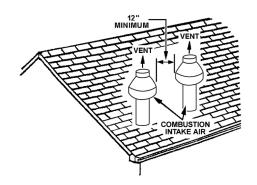
Figure 31: CONCENTRIC VENT TERMINATIONS FOR VERTICAL DIRECT VENTING THROUGH A ROOF
